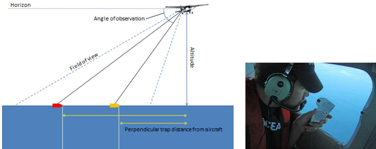
**Figure 3.** Left: Diagram showing how angle of observation can be used to calculate perpendicular distance of buoys from the aircraft transect track line. Right: Observer Dr. Geoff Shester views traps from the window of the aircraft using a clinometer to determine the angle of each observed trap relative to the aircraft.
