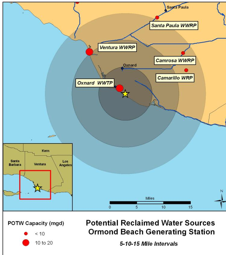
Figure K-6. Reclaimed Water Sources
