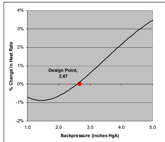
Figure K-11. Estimated Heat Rate Correction (Unit 2)
