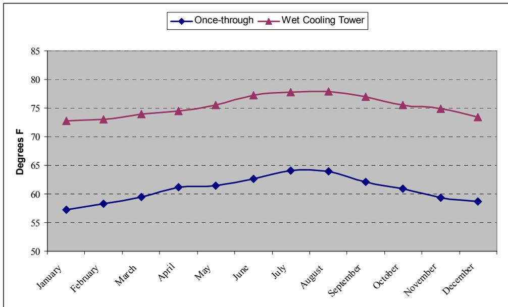
Figure K-7. Condenser Inlet Temperatures
