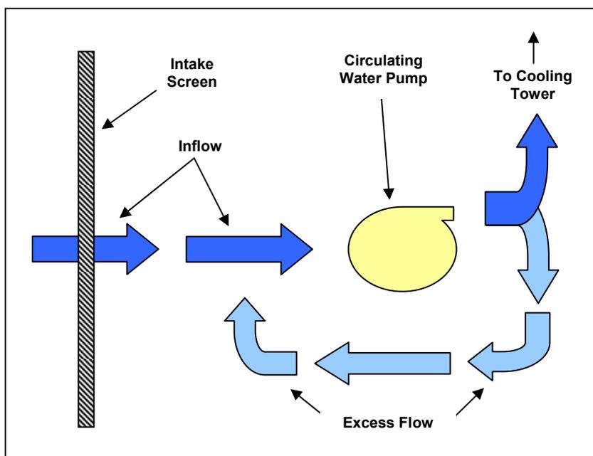
Figure K-5. Schematic of Intake Pump Configuration
