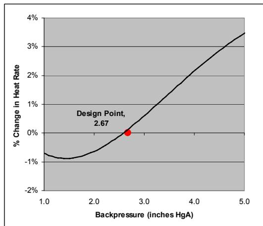
Figure K-9. Estimated Heat Rate Correction (Unit 1)
