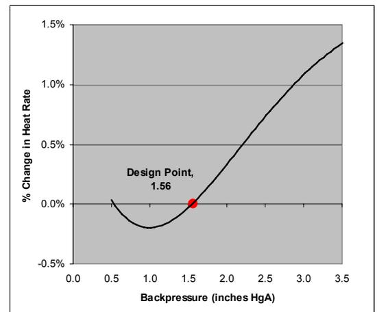
Figure F-14. Estimated Heat Rate Correction (Unit 8)
