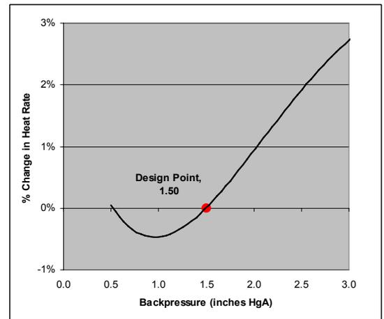
Figure F-12. Estimated Heat Rate Correction (Units 5 & 6)
