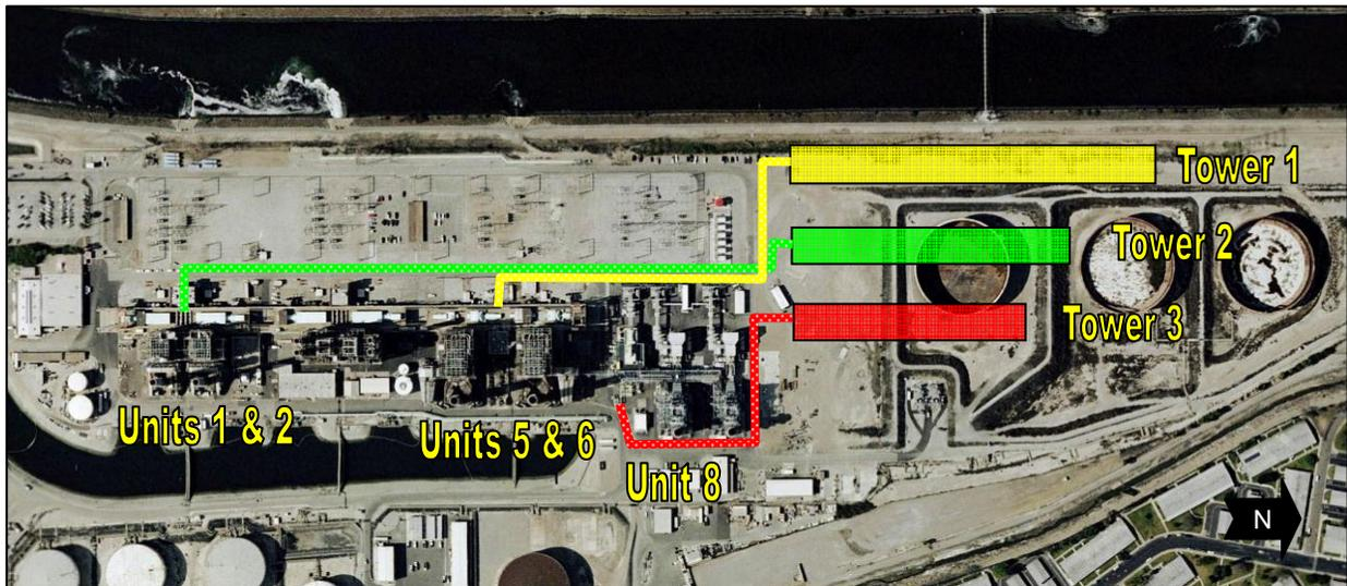
Figure F-5. Location of Cooling Towers and Underground Piping
