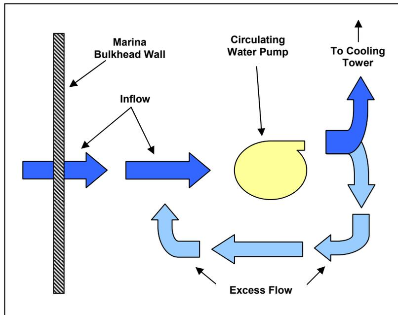
Figure F-6. Schematic of Intake Pump Configuration
