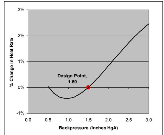
Figure F-10. Estimated Heat Rate Correction (Units 1 & 2)
