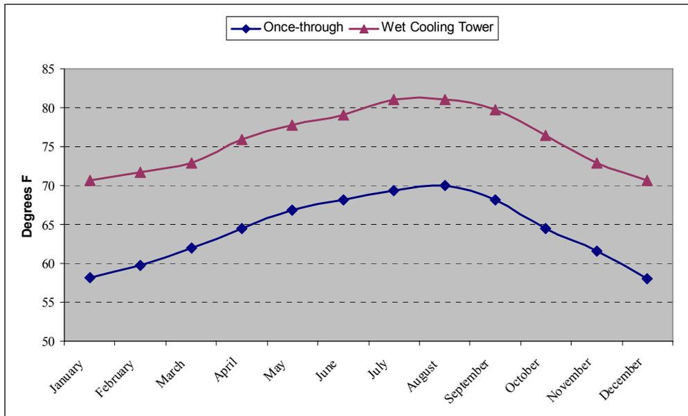
**Figure F-8. Condenser Inlet Temperatures**
