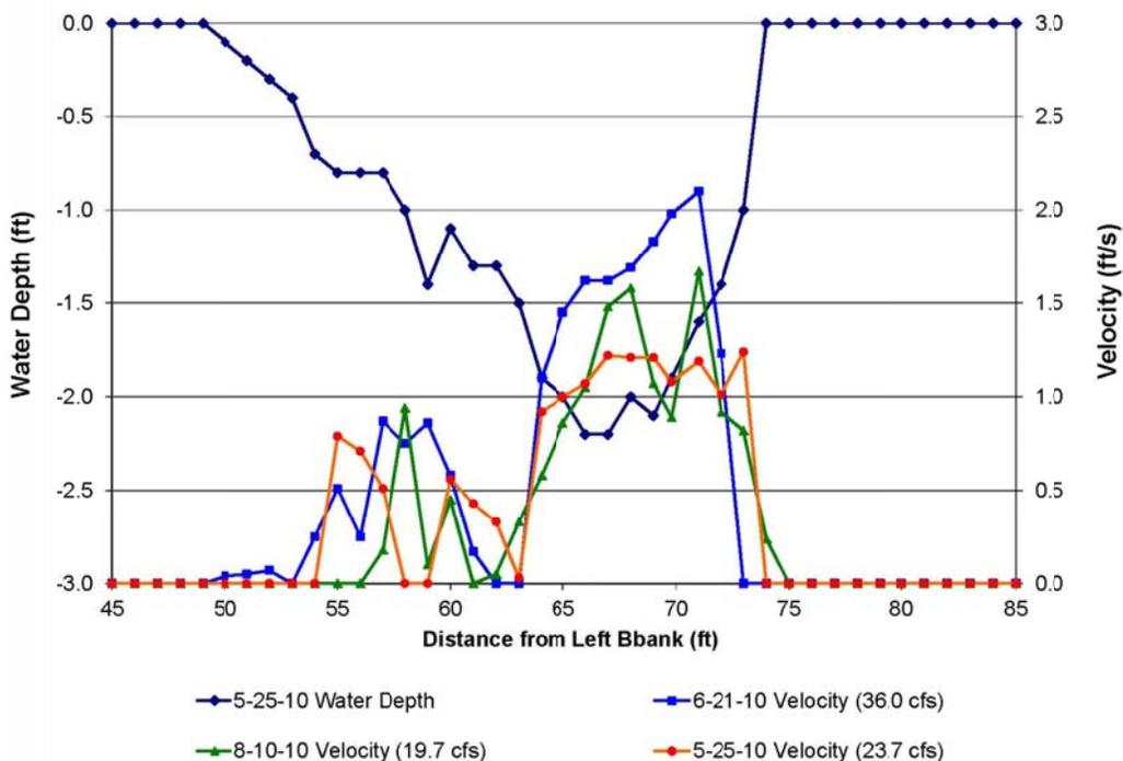
Figure 69. Water depths and average column velocities at TNC Site Pool cross section No.5 at three streamflows.
