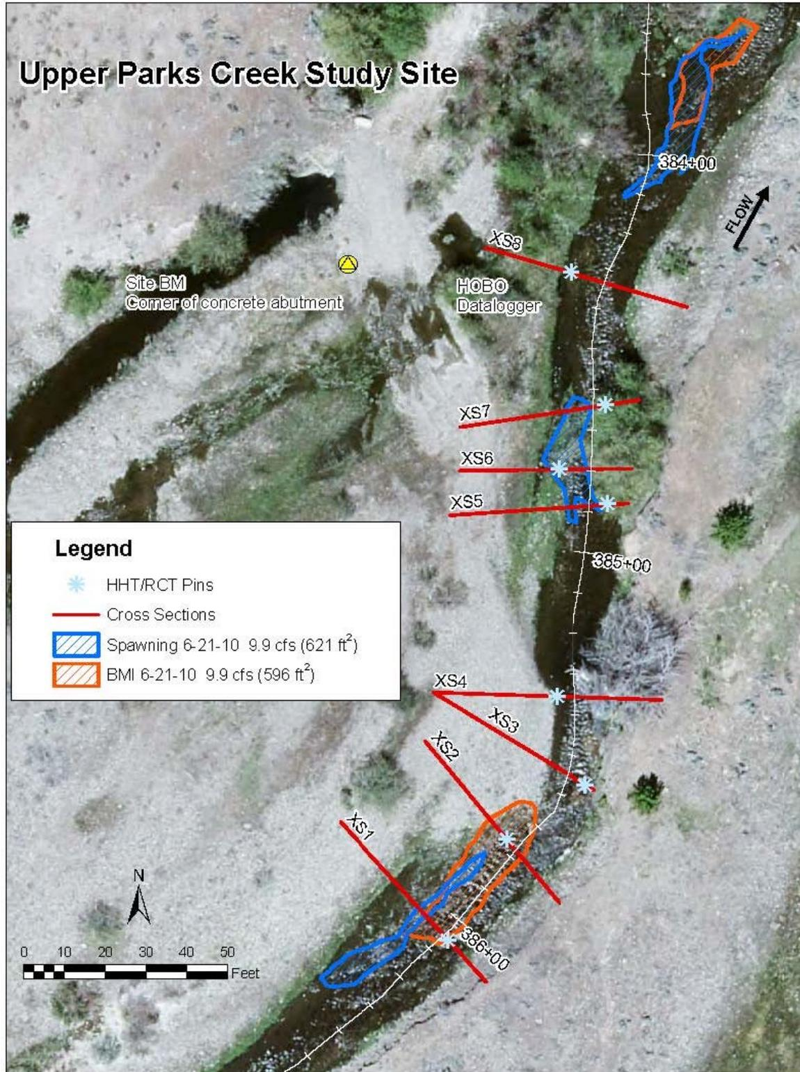
Figure 37. DHM polygons for salmonid spawning habitat and BMI riffle habitat in the UPC study site mapped on June 21, 2010, at 9.9 cfs.
