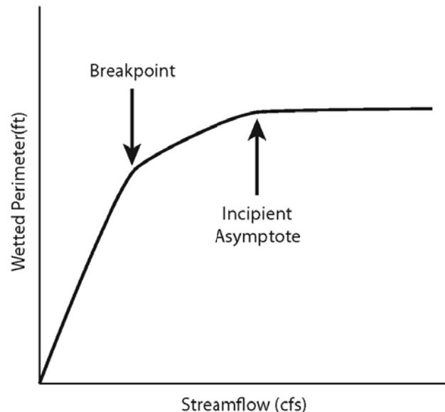
*Figure 4. Wetted perimeter method of selecting the 'Incipient Asymptote' versus the 'Breakpoint' to achieve a more desirable level of habitat protection (CDFW 2011).*
