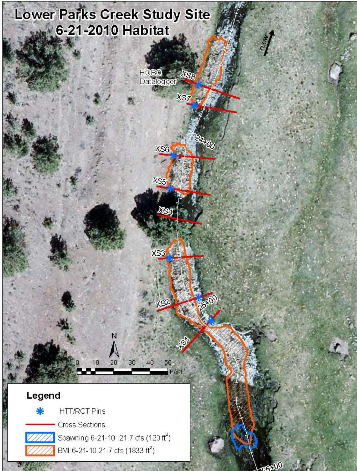
Figure 39. LPC study site with BMI and spawning habitat polygons mapped at 21.7 cfs on June 21, 2010.
