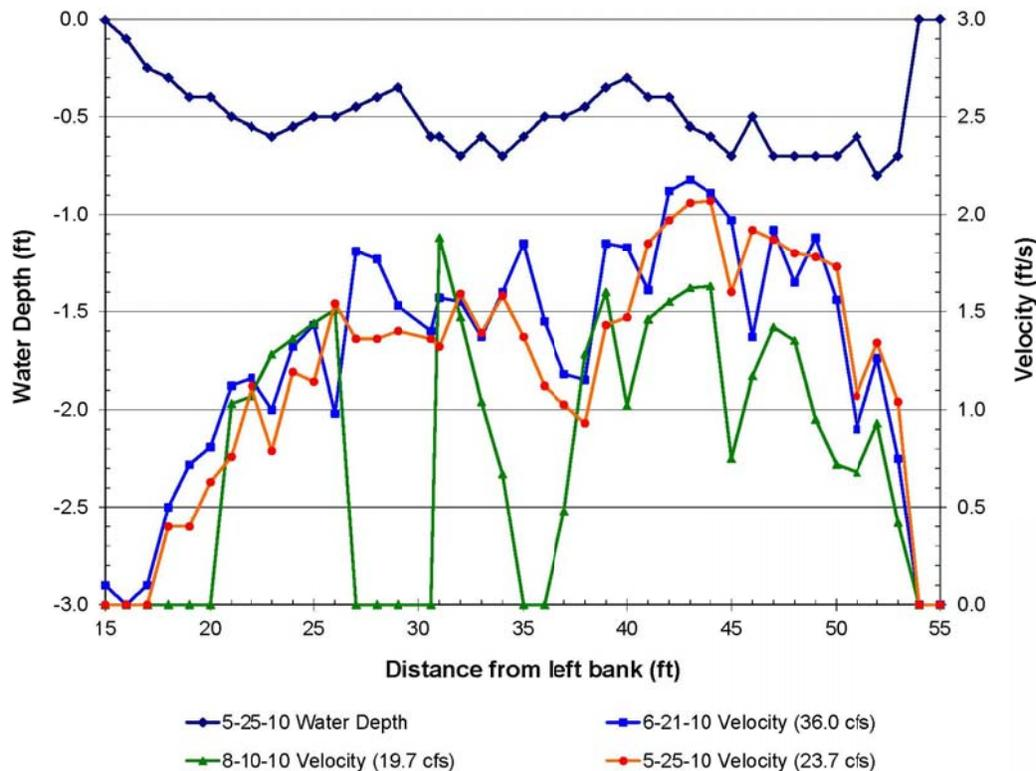
Figure 70. Water depth and average column velocities at TNC Study Site Riffle cross section No.6 at three streamflows.
