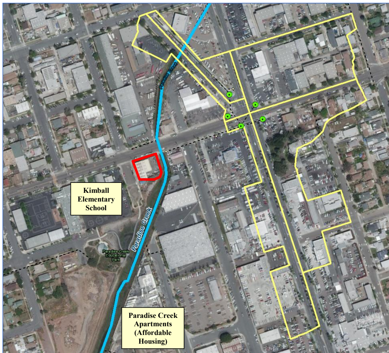
Trash Control BMPs Site Map. Project location (red polygon), storm drain pipes (black dashed lines), five trash control BMP locations (green points), and trash control BMP drainage areas (yellow polygons). The five trash control BMPs drain approximately 15 acres.
