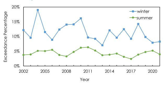
Figure 8. Average Enterococcus Exceedance Rates in California from 2002 to 2021. The exceedance rate for each beach is assessed based on the standards described in 2012 Recreational Water Quality Criteria by US EPA. The bacteria data came from all 17 coastal counties and 27 different monitoring agencies.
