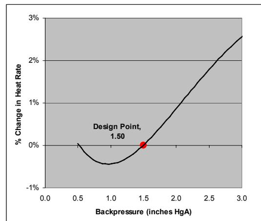
Figure O-10. Estimated Heat Rate Correction (Unit 1)
