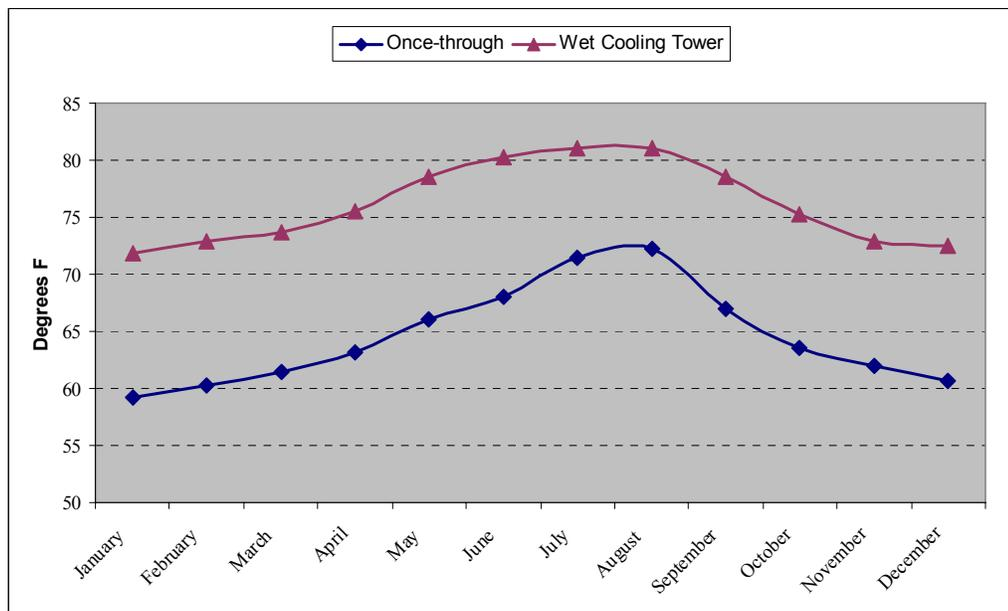
Figure O–8. Condenser Inlet Temperatures
