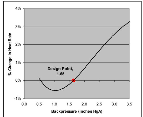
Figure O-14. Estimated Heat Rate Correction (Unit 3)
