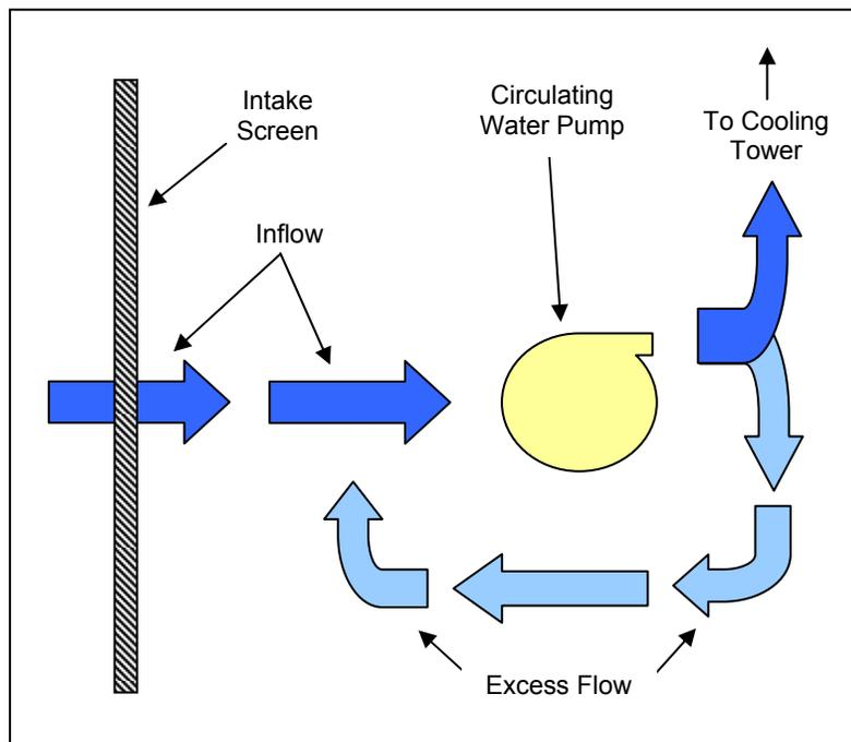
Figure O-6. Schematic of Intake Pump Configuration
