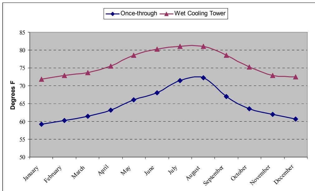
Figure O–8. Condenser Inlet Temperatures
