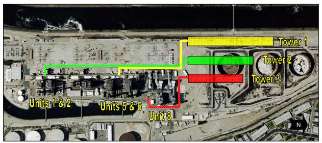
Figure F–5. Location of Cooling Towers and Underground Piping
