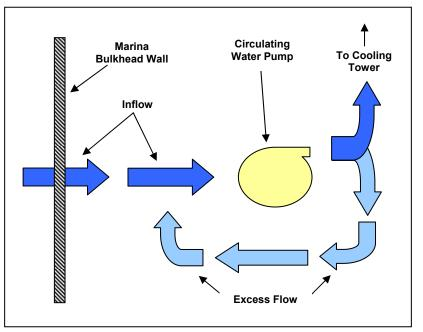
intake of new water, measured at the bulkhead wall in the marina, will be equal to the makeup water demand of the cooling towers. Figure F–6 presents a schematic of this configuration.
