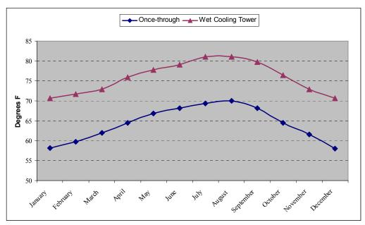
Figure F-8. Condenser Inlet Temperatures
