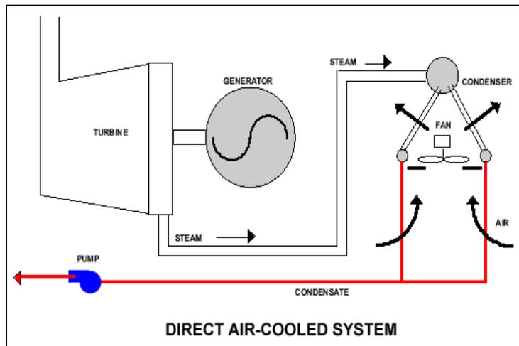
Figure 4-6. Air Cooled Condenser (“Direct Dry”)
