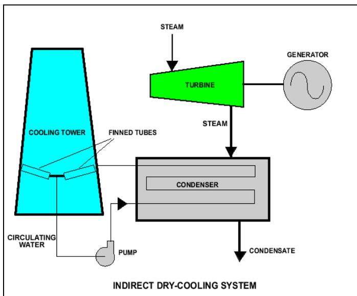
Figure 4-7. Indirect Dry Cooling
