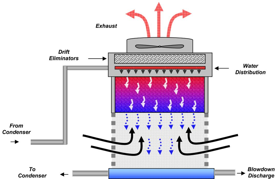
Figure 1-4. Counterflow Cooling Tower
