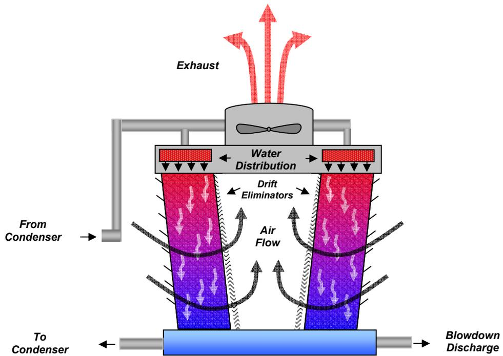
Figure 4-3. Crossflow Cooling Tower
