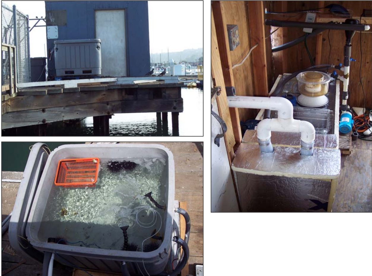
Figure III-D-3 Circulating Sea Water Tank
