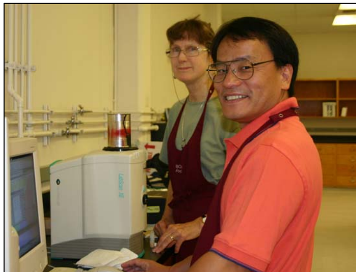
Figure 1. The Hunter Lab Scan color measuring system includes the sea urchin gonad sample, under the can in the middle of the photo, and computer software that gives the color readings. Each gonad sample is scanned three times by the Hunter Lab Scan and the average of those three values gives the sample color in red, yellow and lightness.
